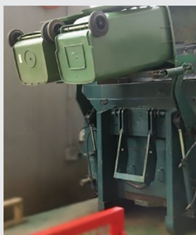
Cleansing workers deposit waste properly wrapped in designated bags into a refuse compaction system
