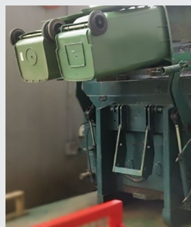
Cleansing workers deposit waste properly wrapped in designated bags into a refuse compaction system
