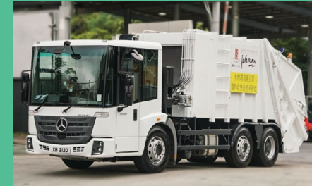
FEHD's contractors' RCVs with rear compactors
