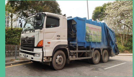
PWC's RCVs with rear compactors
