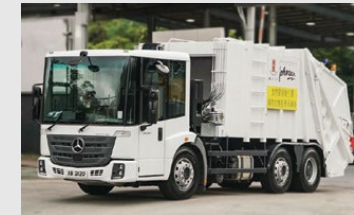
FEHD's contractors' RCVs with rear compactors
