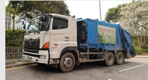
PWC's RCVs with rear compactors
