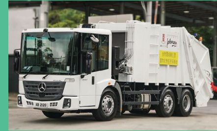
FEHD's contractors' RCVs with rear compactors
