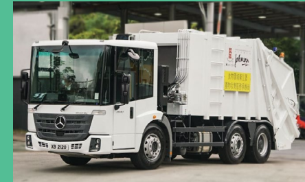
FEHD's contractors' RCVs with rear compactors
