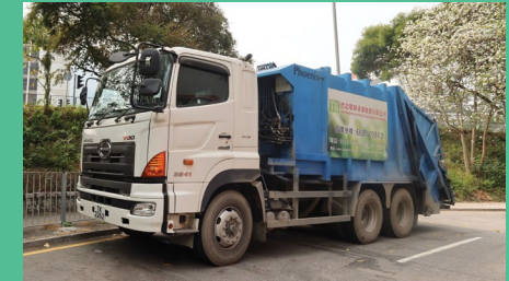
PWC's RCVs with rear compactors
