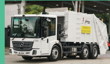
FEHD's contractors' RCVs with rear compactors
