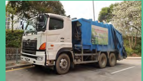
PWC's RCVs with rear compactors
