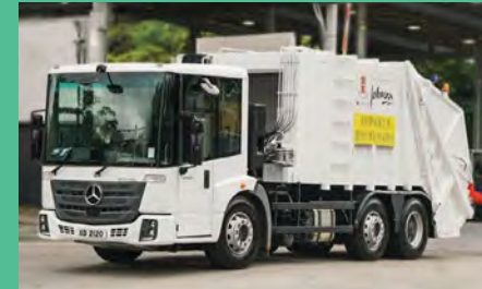
FEHD's contractors' RCVs with rear compactors
