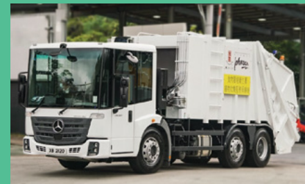
FEHD's contractors' RCVs with rear compactors
