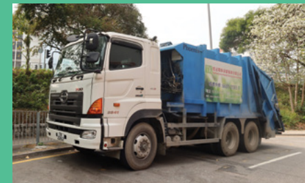
PWC's RCVs with rear compactors
