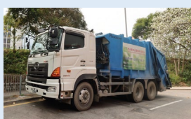
PWC's RCVs with rear compactors
